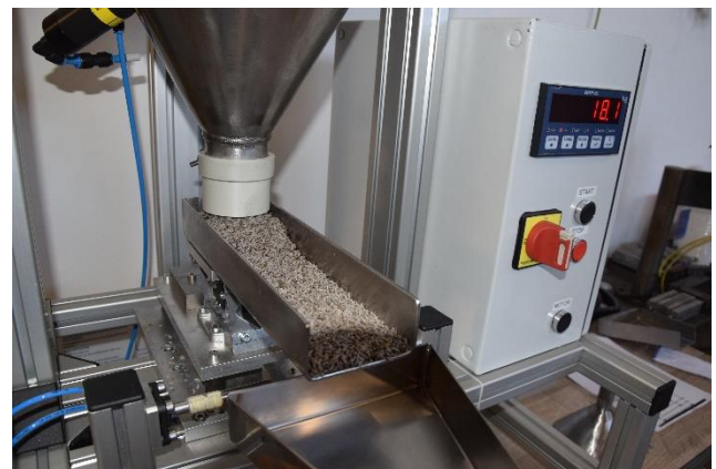
Figure 4. System transport and distribution of material
