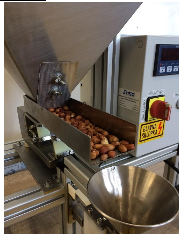
Figure 6. Material transport and distribution system
